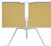
Incorrect installation Too loose pressure plate tube
