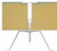
Incorrect installation Too loose pressure plate tube
